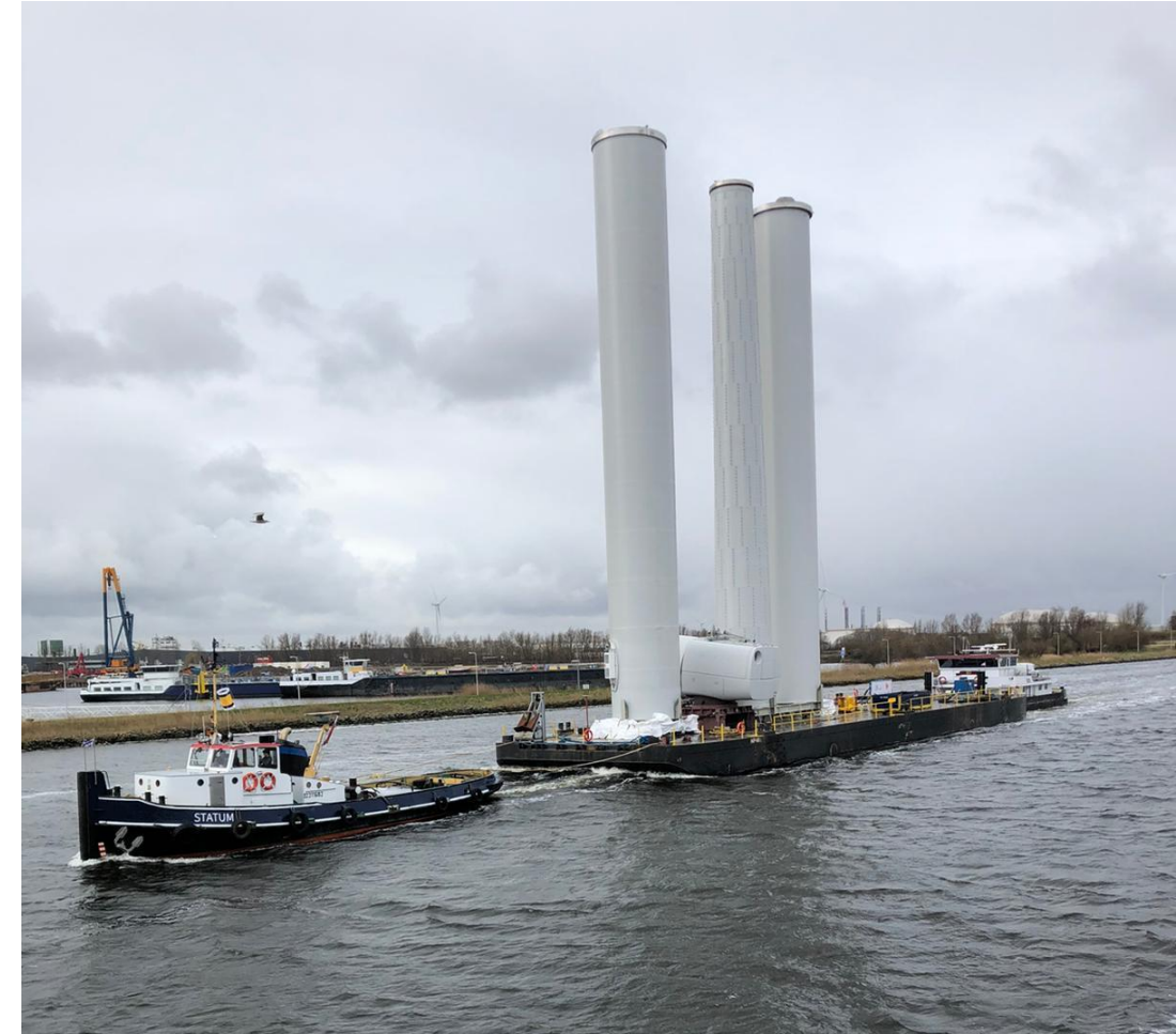
Example bringing components to installation vessel in sheltered locations (Van Oord | Windpark Fryslan)
