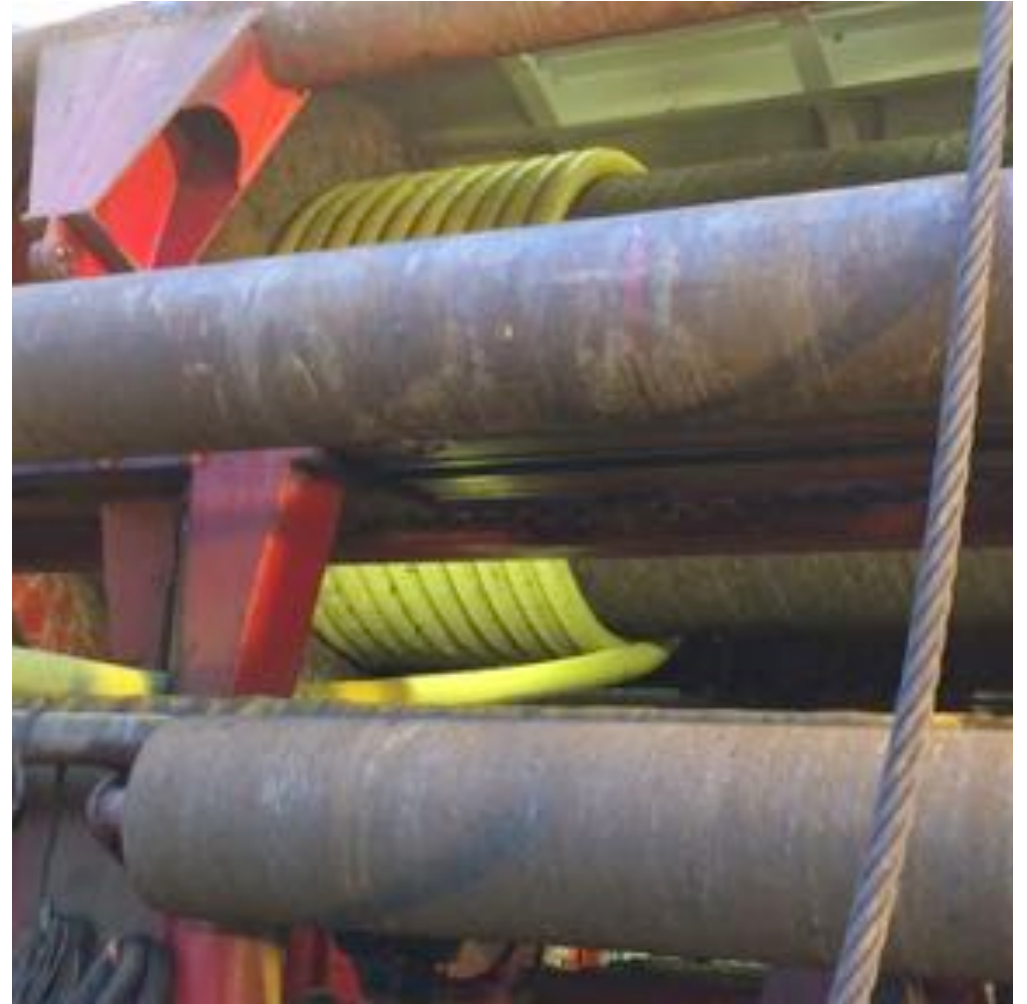
Spooling 200m demonstrator MODU rope with Calorfloat® on Skandi Vega
