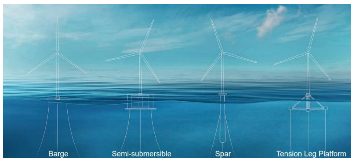
Figure 12: FOW foundation types
